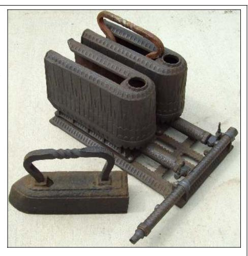
This gas heated tailor's stove and irons are believed to be the first of the type used in Gympie around 1912. The tailor's iron was known as a goose, and these irons are large and very heavy, weighing 20 pounds each (9 Kg).
